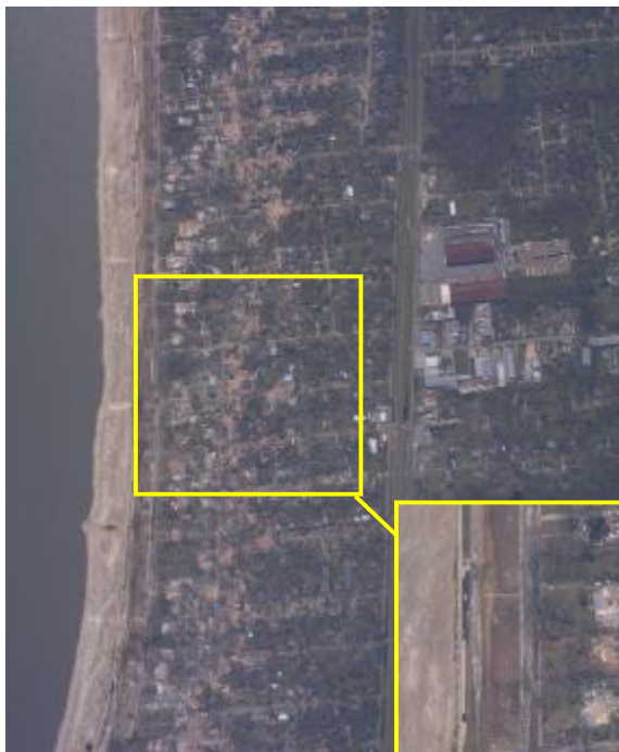
Figure 4: Aerial photographs of damages near Gulfport, Mississippi after Hurricane Katrina [provided by NOAA]. Note the difference in damages in buildings on either side of the debris field. The debris field was created by the storm surge, and those structures impacted by the storm surge were essentially destroyed, whereas buildings inland from the storm surge remained intact.
