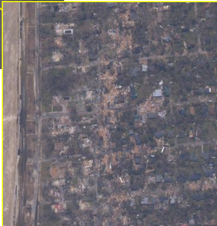
Figure 4: Aerial photographs of damages near Gulfport, Mississippi after Hurricane Katrina [provided by NOAA]. Note the difference in damages in buildings on either side of the debris field. The debris field was created by the storm surge, and those structures impacted by the storm surge were essentially destroyed, whereas buildings inland from the storm surge remained intact.
