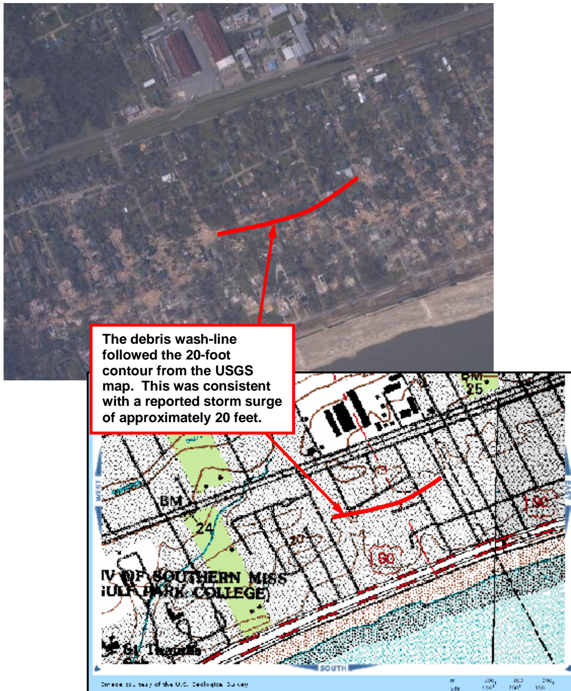
Figure 5: By orienting the NOAA aerial damage photograph from Figure 5 and comparing to a USGS topographic map of the area, the storm surge height may be estimated by examining the location of the debris wash-line.
